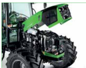
TIER 4 FARMOTION COMMON RAIL TURBO INTERCOOLED DIESEL ENGINE
