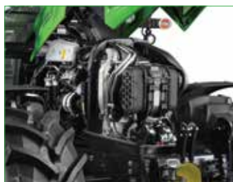
TIER 3 FARMOTION ENGINE 4-CYLINDER TURBO INTERCOOLED
