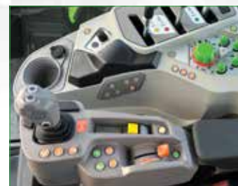
20 SPEED ELECTRONIC ARMREST CONTROLLED FULL POWERSHIFT TRANSMISSION
