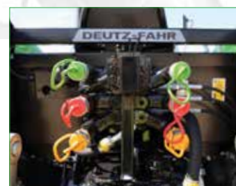
3 STANDARD HYDRAULIC REMOTES WITH ONE MANUAL FLOW DIVIDER
