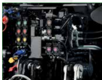
120 L/MIN CAPACITY CLOSED-CENTRE HYDRAULIC SYSTEM
