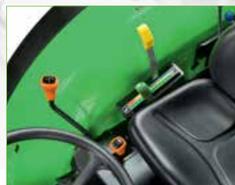
WET CLUTCH POWER SHUTTLE WITH 3-STAGE ECO-SPEED POWERSHIFT TRANSMISSION (45X45)
