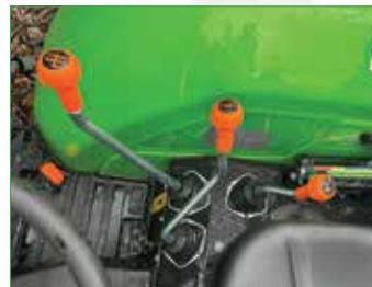
3-RANGE 15F/15R SYNCHROMESH TRANSMISSION WITH A HEAVY-DUTY 11" DUAL DRY CLUTCH FOR SMOOTH OPERATION
