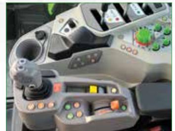
20 SPEED ELECTRONIC ARMREST CONTROLLED FULL POWERSHIFT TRANSMISSION
