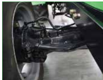
FRONT AXLE BRAKES WITH 4WD BRAKING FOR IMPROVED SAFETY, TRACTION AND REDUCED BRAKE WEAR
