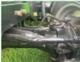
OIL-IMMERSED DISC BRAKES ON ALL FOUR WHEELS
