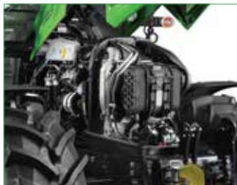
TIER 3 FARMOTION ENGINE 4-CYLINDER TURBO INTERCOOLED
