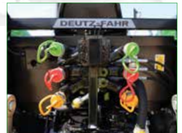
3 STANDARD HYDRAULIC REMOTES WITH ONE MANUAL FLOW DIVIDER
