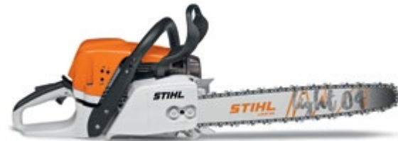
MS 311 PETROL CHAINSAW 59.0CC • 3.1KW • 6.2KG* • 50CM/20"
