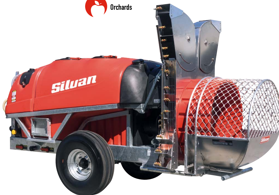
Pictured: 3400L unit with Radak conveyor and optional leaf guard
