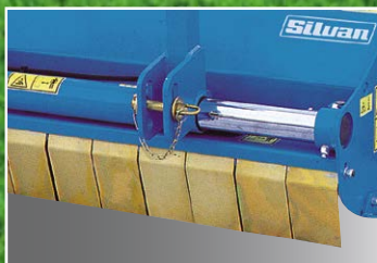
Hydraulic and manual side-shift options
