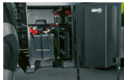
The battery and a tool storage compartment are handily located in the access steps on the right-hand side.
