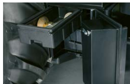
The battery and a tool storage compartment are handily located in the access steps on the right-hand side.
