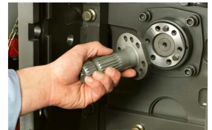
The PTO stub can be changed easily.
