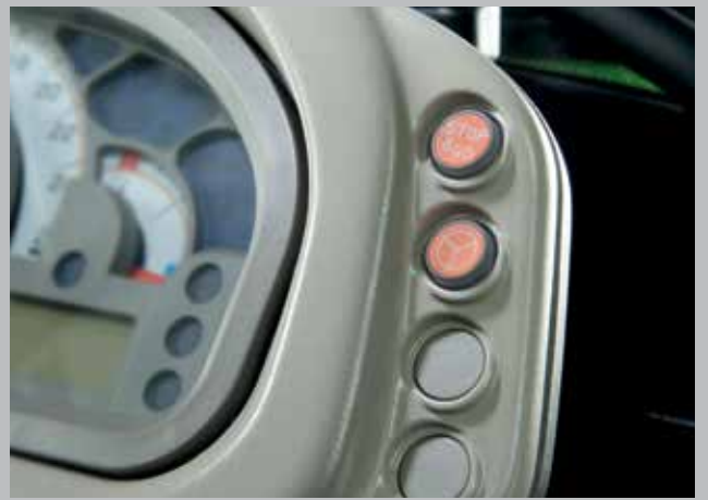
Push buttons to activate the Stop&Go and SDD functions.
