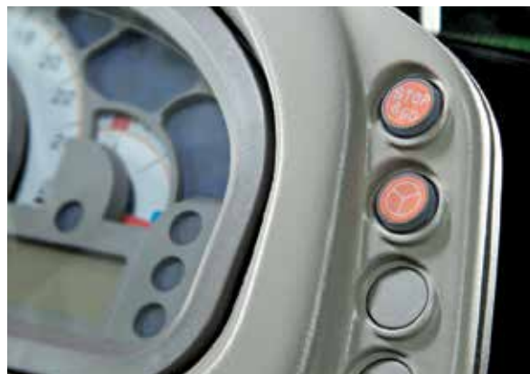
Stop and Go activation via push button.
