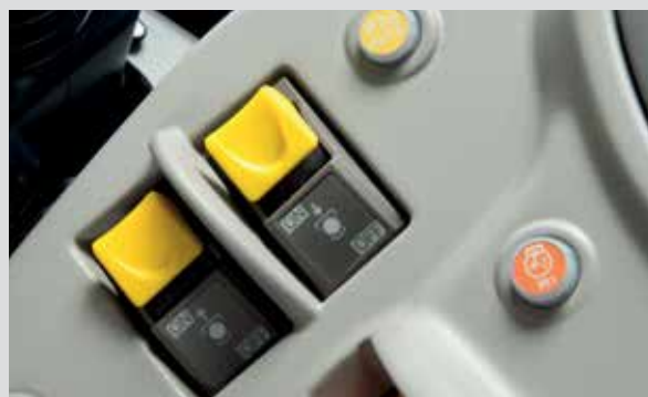
Electro-hydraulic switches to engage PTO.
