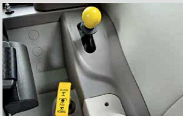
Easy mechanical PTO speed engagement.
