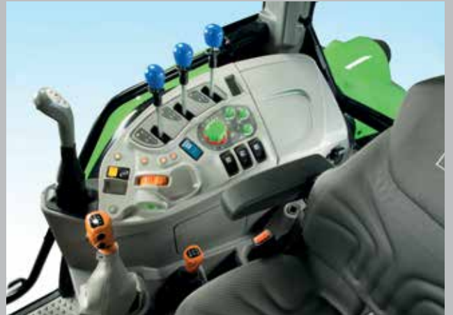
The loader control joystick integrates perfectly in the right-hand console.
