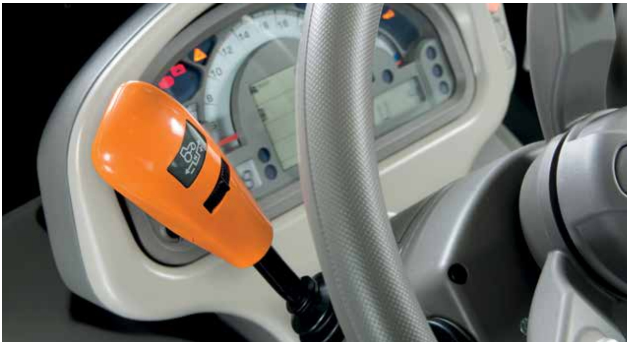
The hydraulic shuttle lever has a useful modulation control function to change reaction time to a change of direction. The roller wheel can set 5 different levels of speed sensitivity.
